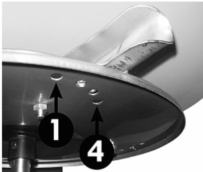
*Spreading disc's vanes regulation*
