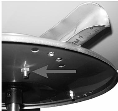
Unscrew the nut and replace the damaged vane.
