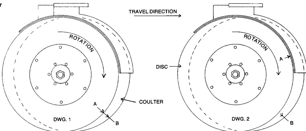
One complete turn changes points A and B (DWG. 1) the amount shown in DWG. 2. It takes 6 turns to bring points A and B back together.
